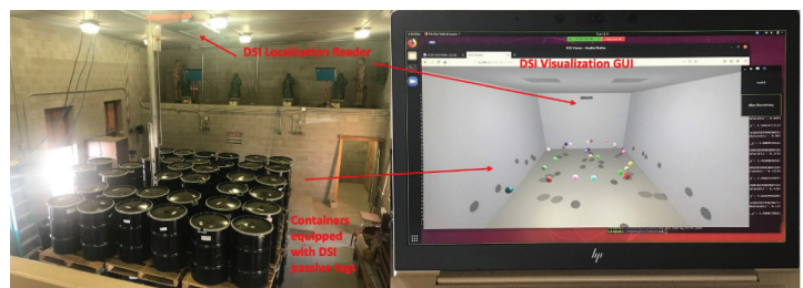
Accurate Asset Localization with < 10 cm Accuracy Using Battery-Free Passive Tags
